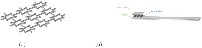
Fig 4. Nine star-shaped auxetic microstructure; (a) 3-D view, (b) As a spacing layer between beam and piezo (Exploded view).
