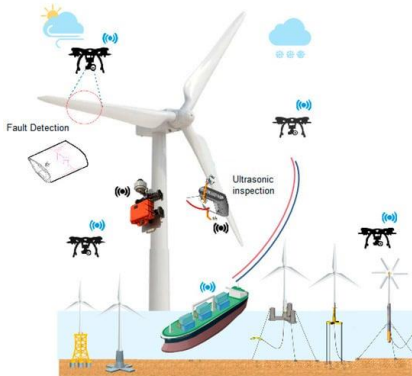
Fig. 1 Concepts of drone/robot outside inspection robot [2]
